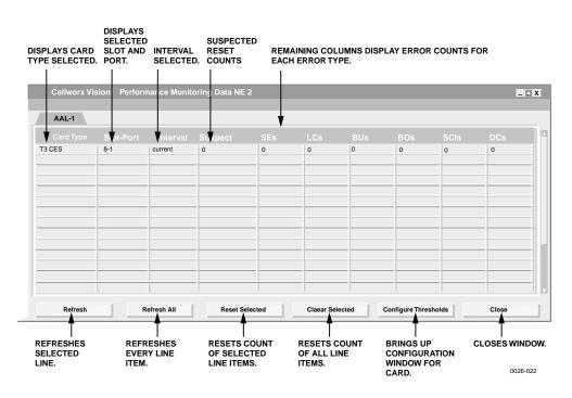
Figure 794-2. Performance Monitoring Data T3 CES Port Window
